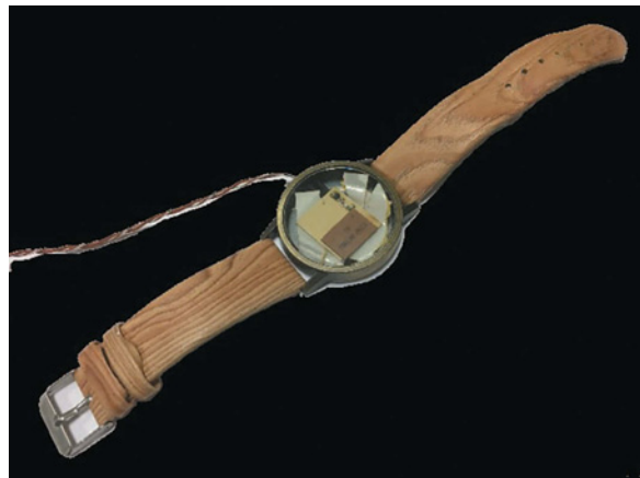
Figure 7. The backscatter modulator embedded into a watch.
